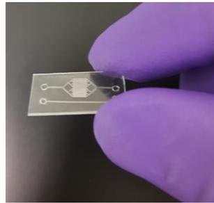
Multiple channel microfluidic COC Device.
