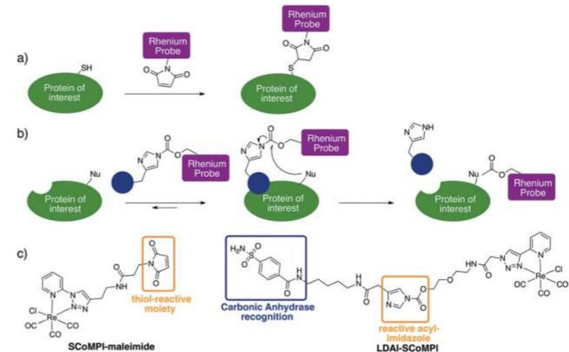
Fig. 1 Labeling of proteins with SCoMPI for X-ray fluorescence imaging. (a) Labeling of an exogenous protein using the thiol-maleimide reaction. (b) Labeling of an endogenous protein using the "Ligand-Directed Acyl Imidazole" chemistry. The blue circle represents a ligand of the protein. (c) (left) Structure of SCoMPI-maleimide for the *in vitro* labeling of homeodomains and (right) structure of LDAI-SCoMPI for the labeling of endogenous carbonic anhydrases.
