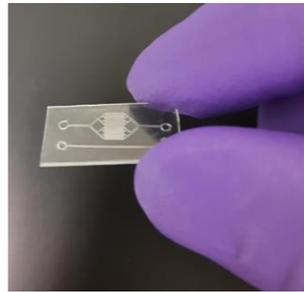
Multiple channel microfluidic COC Device.
