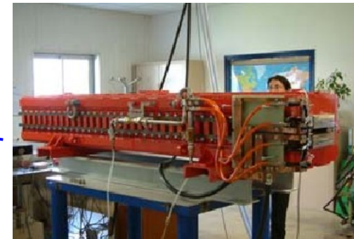
Dipole for electron beam deviation ( www.synchrotron-soleil.fr )
