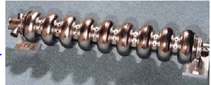
RF cavity electron beam acceleration ( www.synchrotron-soleil.fr )
