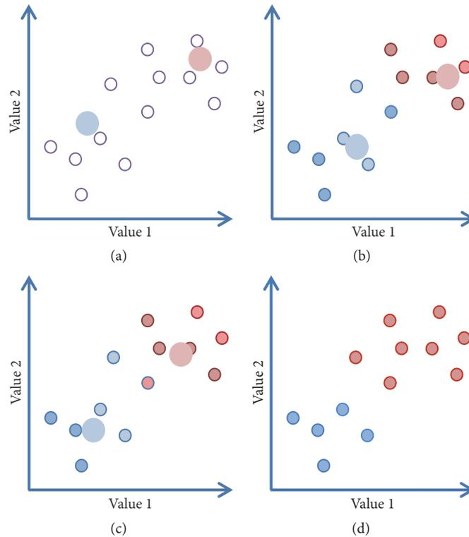
FIGURE 8: *K-Means Clustering*. (a) Two initial seeds are randomly placed within the data. (b) Step 2 indicates positions of the averages of images that are nearest to the seeds. (c) The averages are then recalculated based on the assignments in step 2. Steps 2 and 3 are reiterated; (d) shows the final classes.
