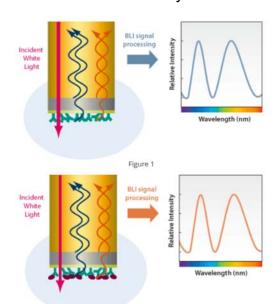
Bio-Layer Interferometry (BLI) is an optical analytical technique that analyzes the interference pattern of white light reflected from two surfaces: a layer of immobilized protein on the biosensor tip, and an internal reference layer.
