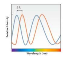
The binding between a ligand immobilized on the biosensor tip surface and an analyte in solution produces an increase in optical thickness at the biosensor tip, which results in a wavelength shift,  $\Delta\lambda$ , which is a direct measure of the change in thickness of the biological layer.
