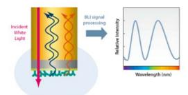
Bio-Layer Interferometry (BLI) is an optical analytical technique that analyzes the interference pattern of white light reflected from two surfaces: a layer of immobilized protein on the biosensor tip, and an internal reference layer.
