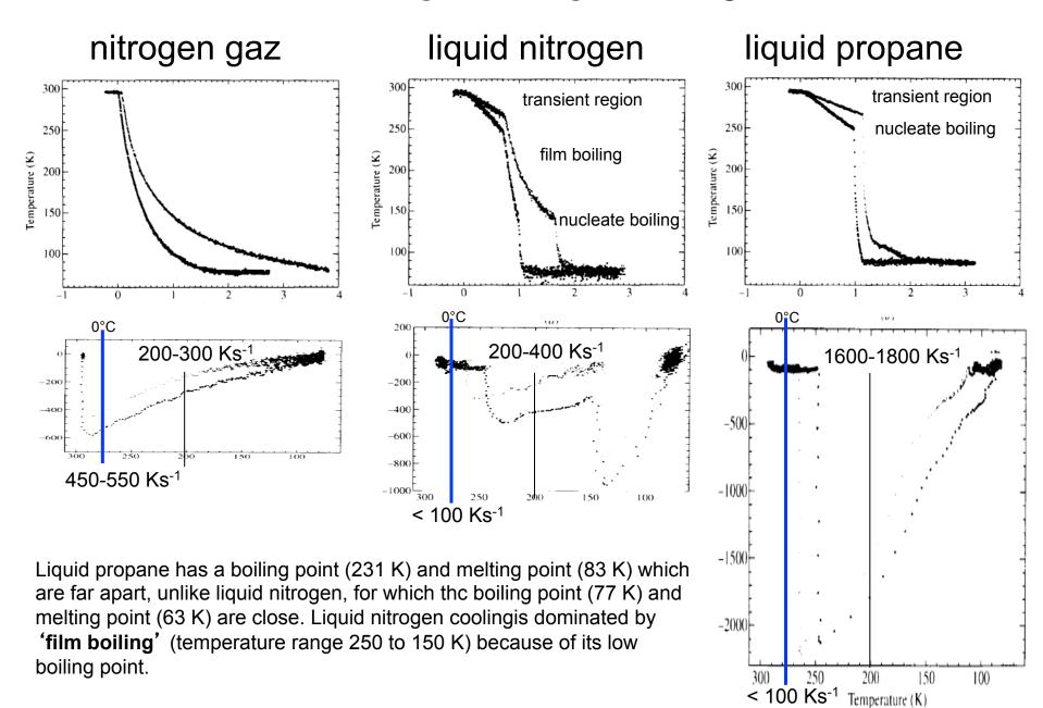
**Cooling Rates During Flash Cooling**
