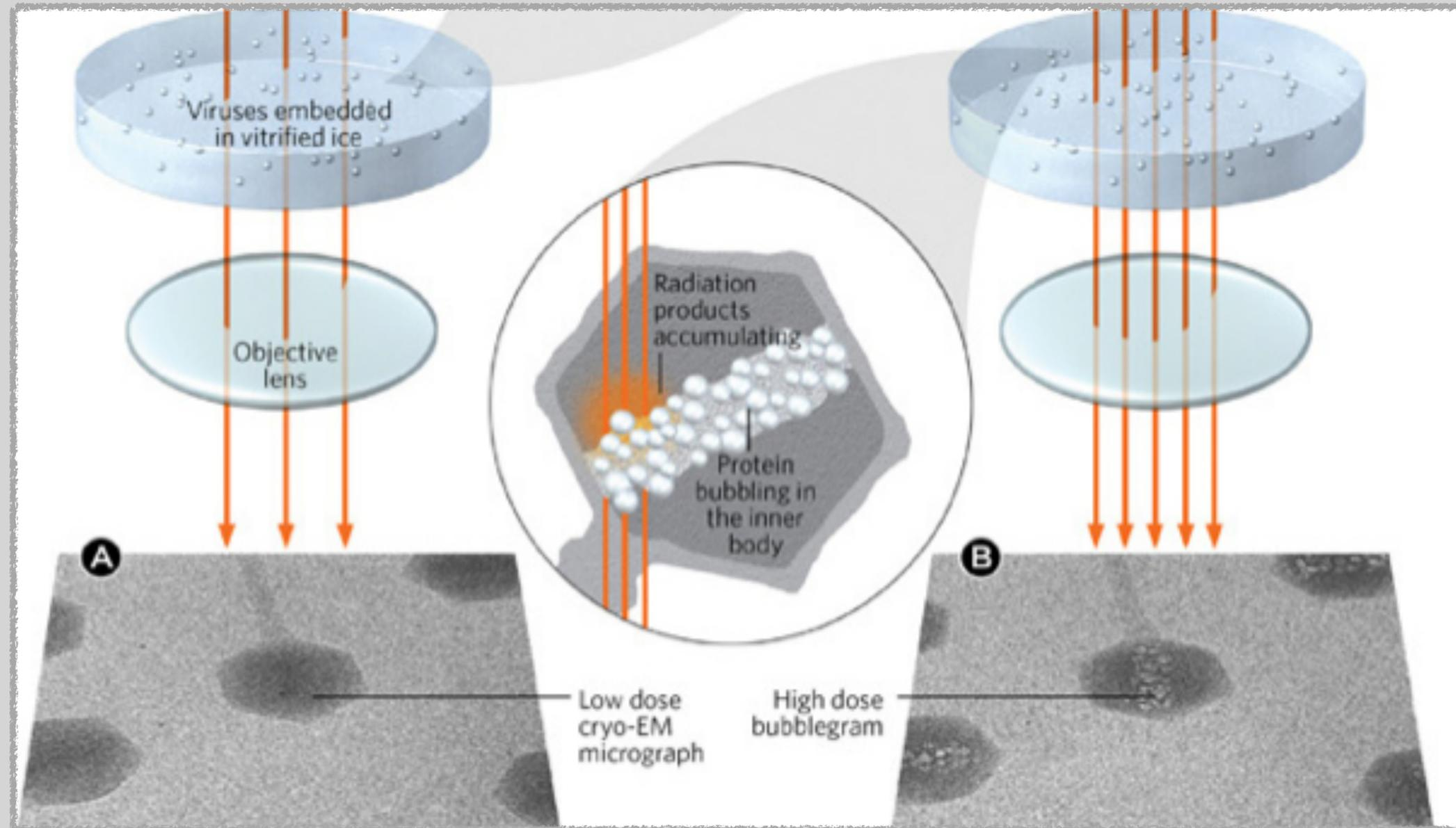
**Frozen samples suffer from radiation damage**
