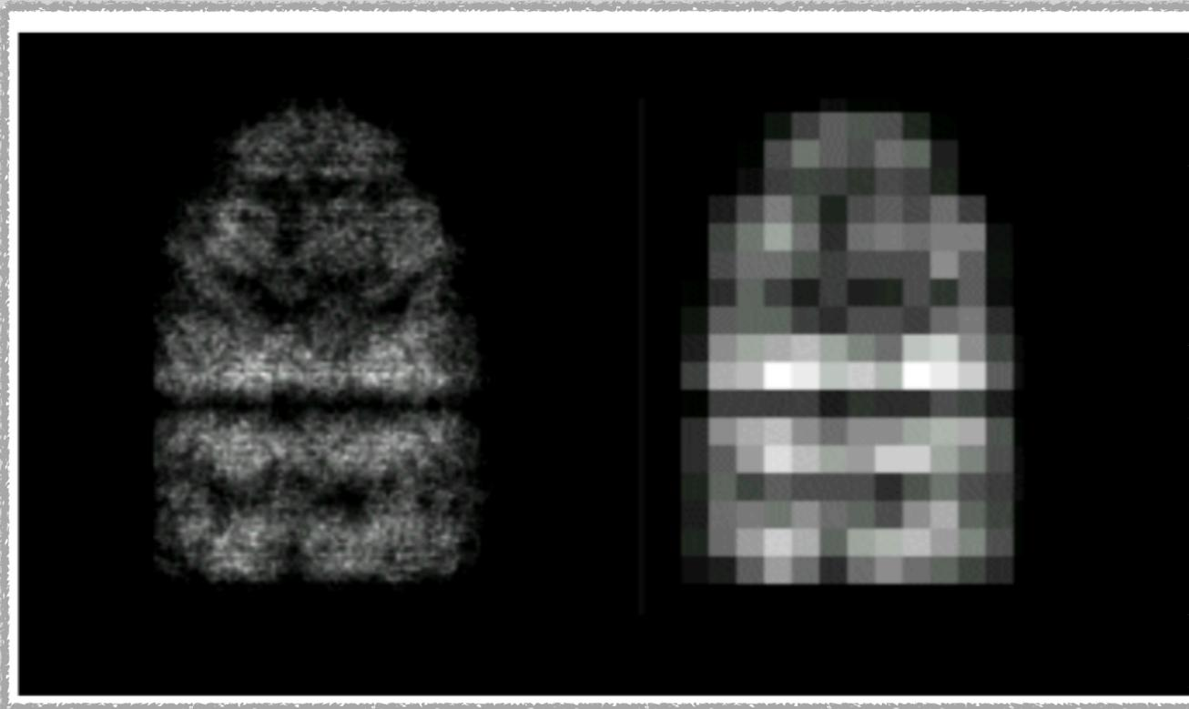
The image is divided up into pixels with a given sampling that determines the highest resolution to analyse.
