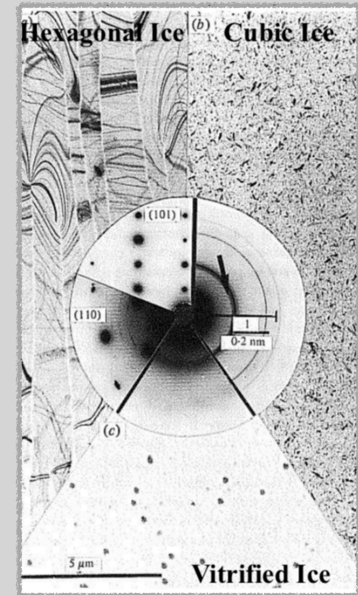
✱✱ Flash-freezing traps biological samples in a vitreous, amorphous ice close to their native state ✱✱
