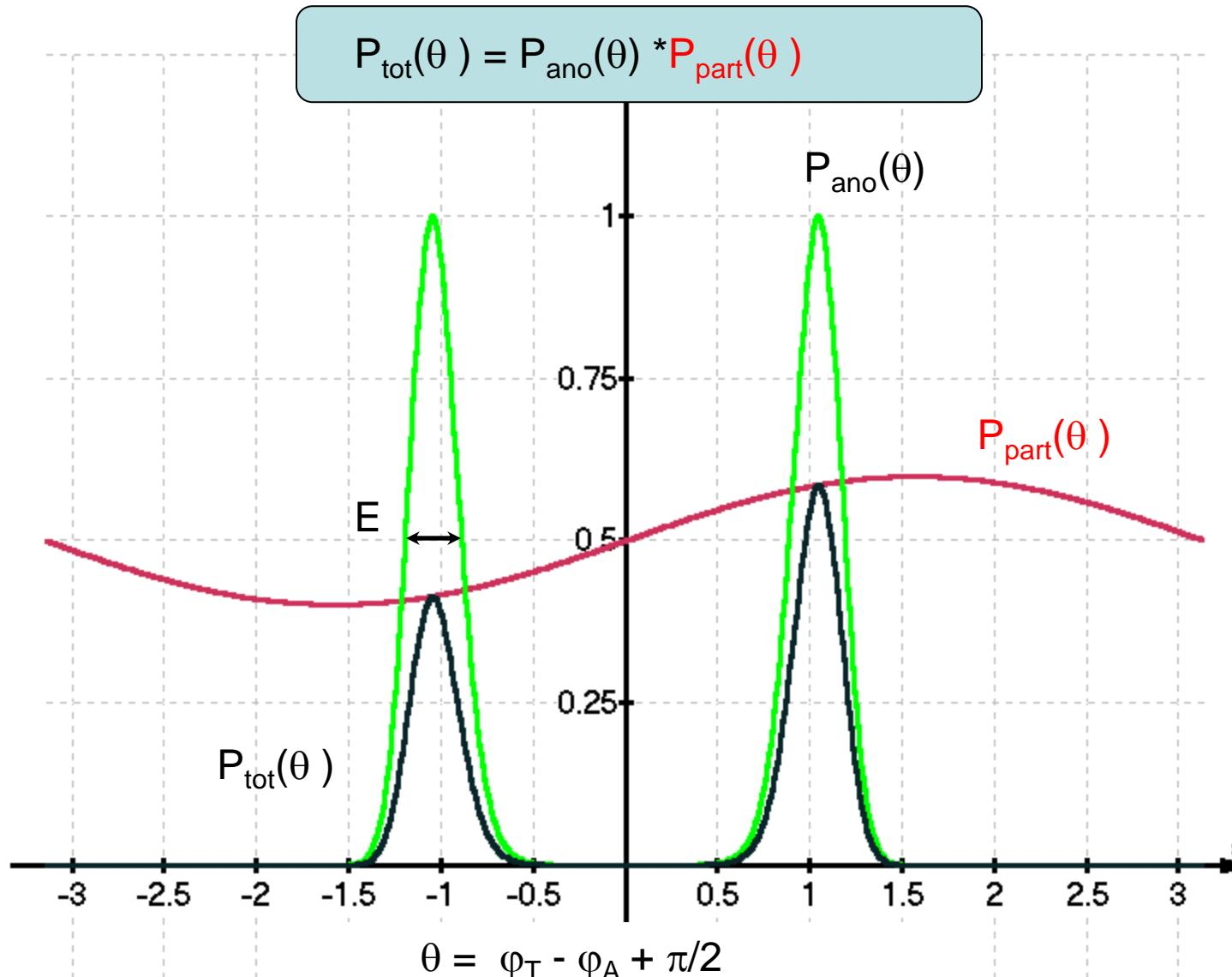
The crystallographer may take the **mean** of the two possible phases and use this along with a weight:  $F = w |F_P| \exp(i\phi_{\text{mean}})$  and then use solvent flattening
