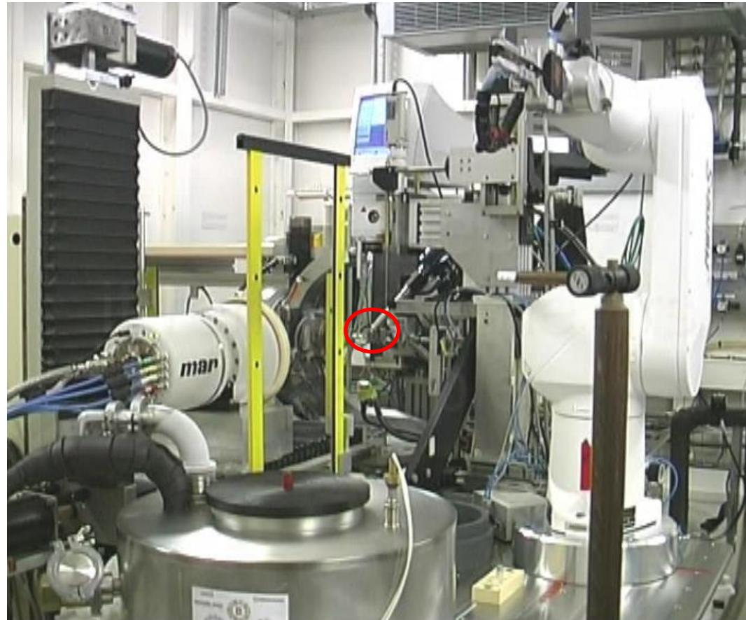
Automated crystal mounting at the ESRF beamline **FIP BM30A**, Grenoble
