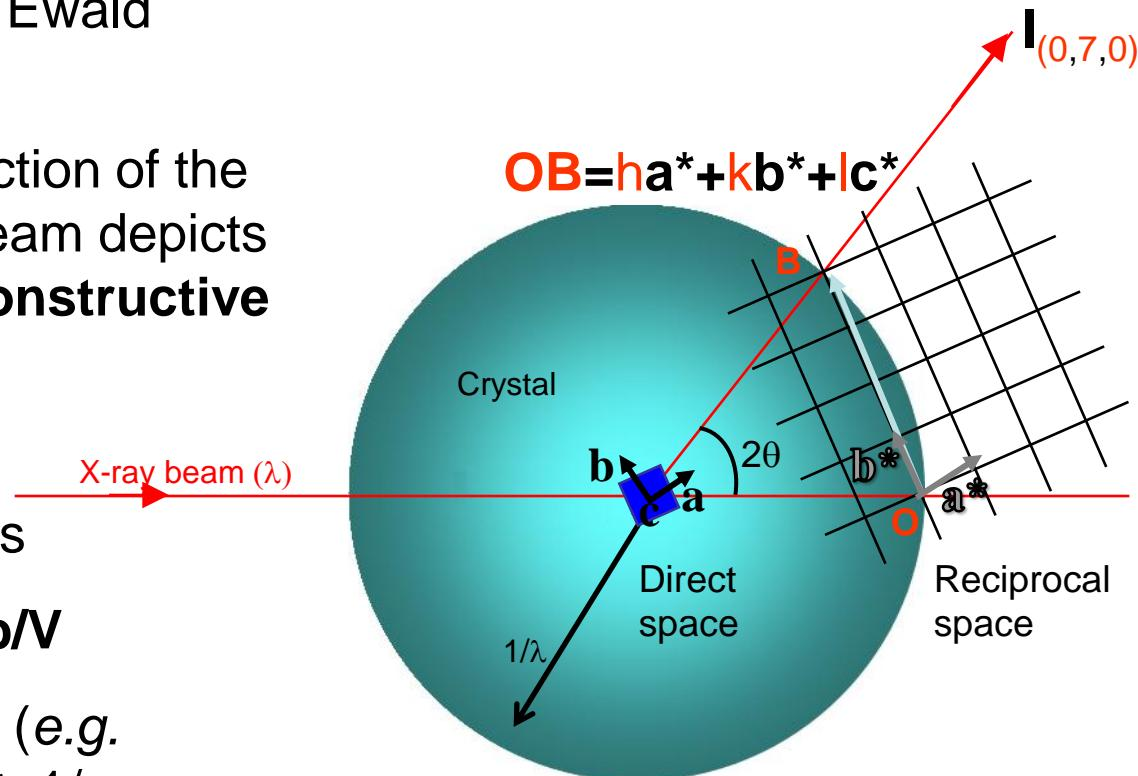
A wave is scattered in a direction **OB** and with a  $2\theta$  angle when a node of the **hkl** grid intersects with the Ewald sphere.
