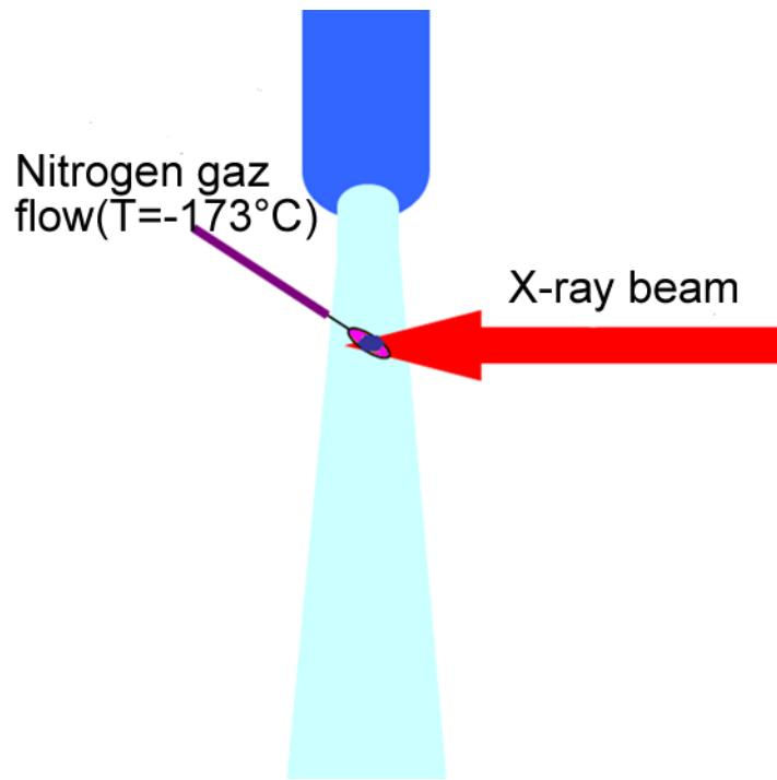
**Crystal fishing** with a cryo-loop and **freezing** to preserve the crystal (dehydration, radiation damage)
