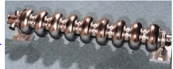
RF cavity electron beam acceleration ( www.synchrotron-soleil.fr )
