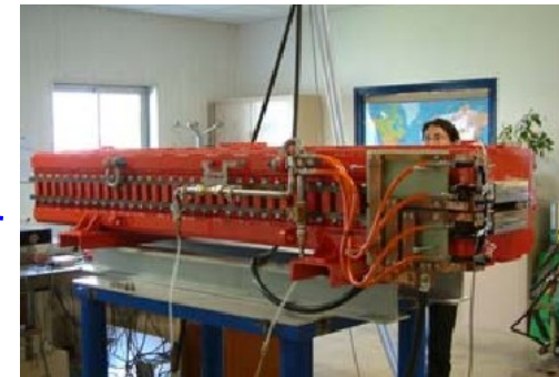
Dipole for electron beam deviation ( www.synchrotron-soleil.fr )
