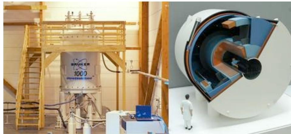
High-resolution superconducting magnet
